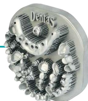
LMP-100 laser printer for most metals is indispensable everywhere, where you need elaborate forms, complex designs and structures, unique products or small series of metal parts. Designed specifically for prosthetic use in dental, but usable in every industry from aeronautics to jewellery. Robust and modularly composed of standard industrial components. Designed to fit it in any lab, enter through each door and drive with a conventional elevator.
